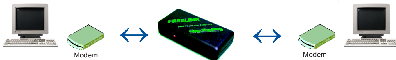
Typical application: The Freelink Demo simulates the analogue connection between 2 modems.
