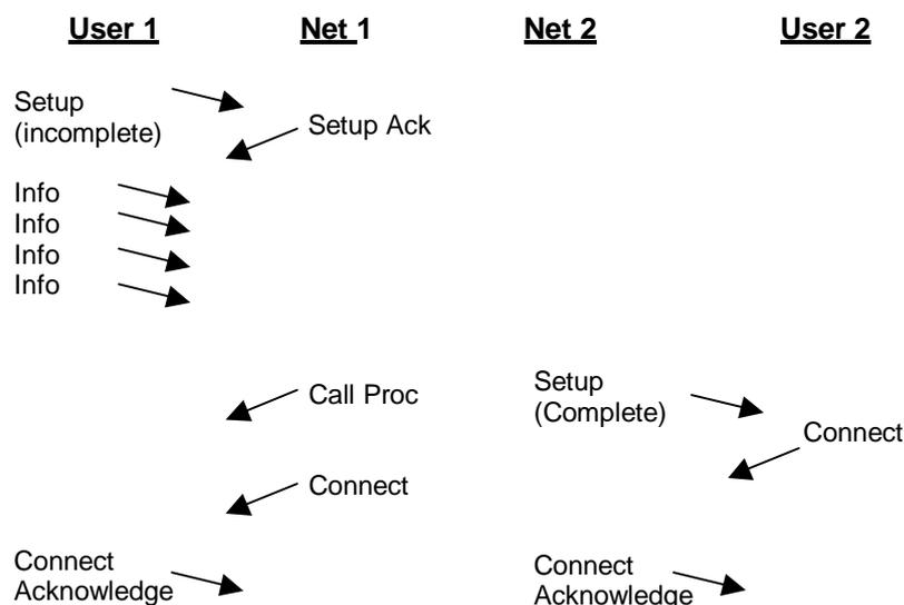
User 1 goes off hook which causes a SETUP message to be sent to Network port 1. This SETUP is incomplete since it does not contain any dialled digits so the network simply responds with a SETUP ACKNOWLEDGE message.
