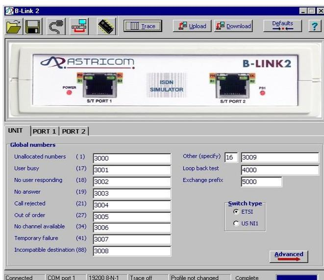
Once a B-Link is found it's front panel image will appear in the main B-Link window and the pop up window will confirm the upload from the B-Link. Click **OK** to access the software which opens in the **Unit** tab showing settings common to all ports. To access settings and advanced features unique to a port click on the appropriate **Port** tab.
